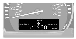
The displays shown in the illustration appear for a few seconds once the ignition key is in position 1 or after starting the engine.
